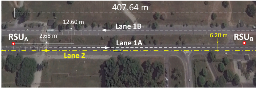
Fig. 8. Experimental scenario used for CooPS evaluation performance. Three separate road stretches were used, Lanes 1A, 1B, and 2. We used two fixed road-side units: RSU_A and RSU_B (figure produced using Google Earth).
